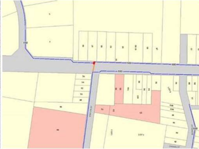
Build 2 - DN150 water main crossing Maitland St between two DN100 mains, near Lot 2//1094098
